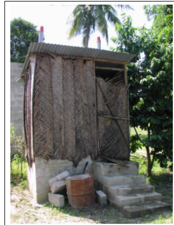
Photo 5: EcoSan toilet with thatch superstructure
